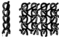
FIG. 2.—A Single Thread formed into a Chain of Crochet Work, showing the Loop Structure of the plain Warp-knitted Fabric. It is built up as shown in the diagram by a number of threads running up the fabric.
